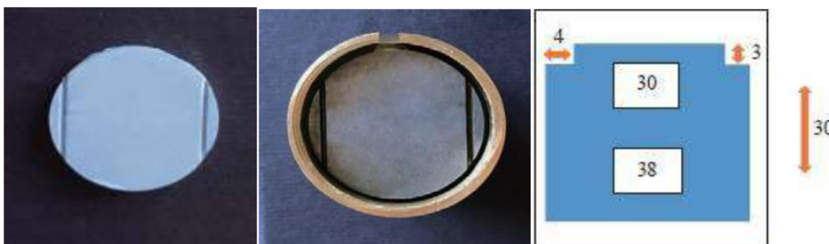
Fig. (1). A teflon mold for dimensional change test.
