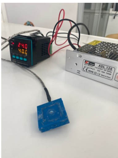
Fig. (1). The temperature measurement device -temperature-sensing metal probe- digital display.
