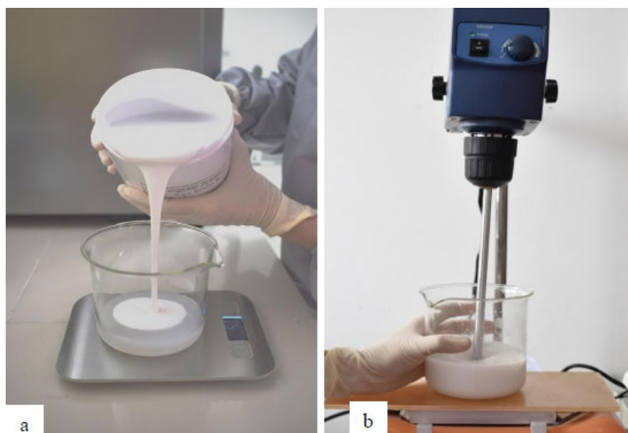
Fig. (2a). Steps for measuring base and RTV silicone catalyst P25 at a ratio of 1:1 using a digital scale. b) The silicone mixture was homogenized using a mechanical mixer at 800 rpm for 3 minutes.
