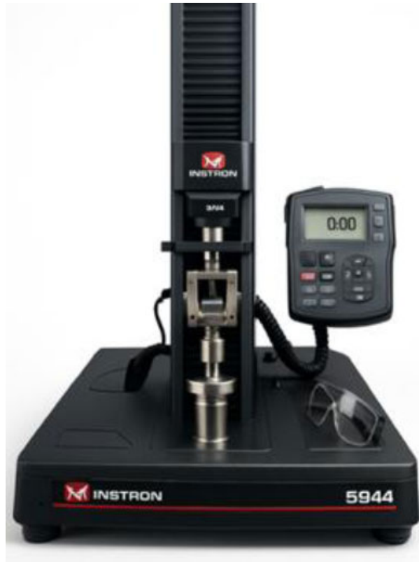
Fig. (4). Testing of specimens was performed using a universal testing machine (Instron 5944, Norwood, MA, USA) equipped with a 2 kN load cell to conduct pull-out tests for evaluating the retention strength of the tested materials.
